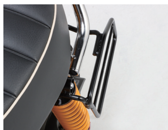
Approximately 24mm of clearance between the side bag support and the rear shock absorber.
